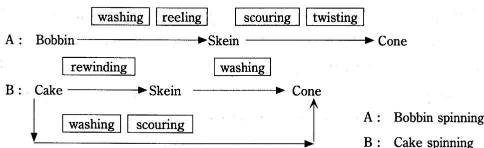
Fig. 4 After-treatment of viscose filament yarns
