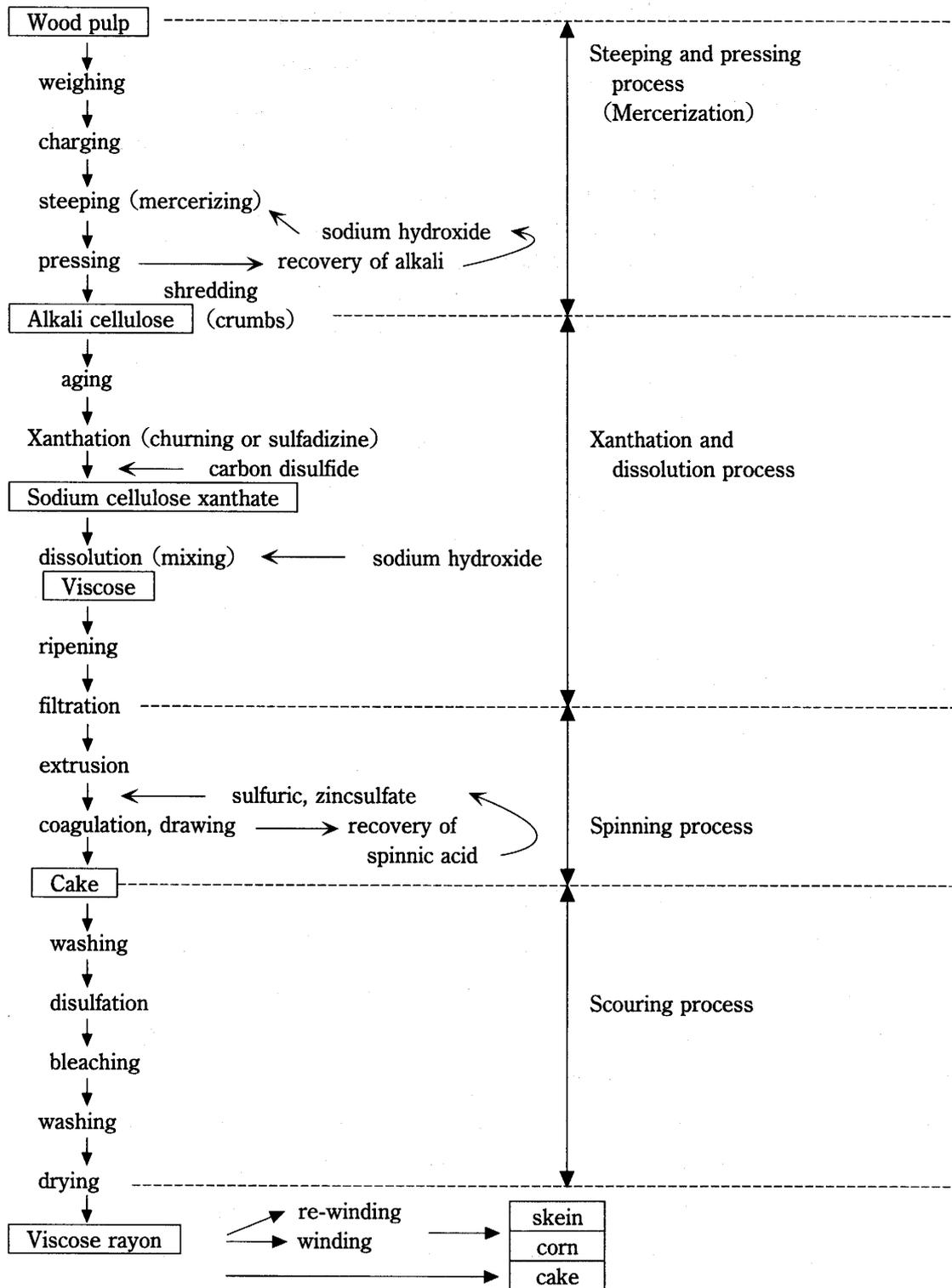
Fig. 2 Manufacturing process of viscose rayon
